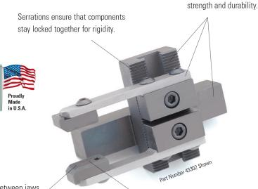
Unit is very easy to use — simply set gap between jaws 1/8" smaller than stock size. As the bar puller slides over the bar along the x-axis, the fingers flex to provide the gripping force. The turret then retracts along the z-axis, pulling the bar out the desired position.
